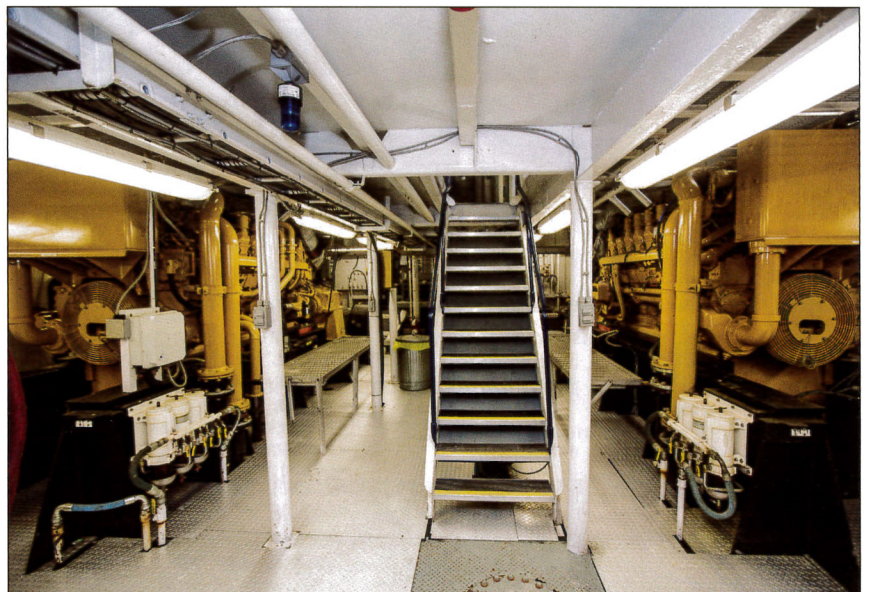
The American Pharoah is powered by twin Cat 3516 diesels.
